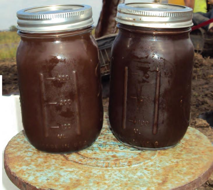
**These pint jar samples were collected during the pigging process show the degree of iron and manganese removed from the pipeline.**
