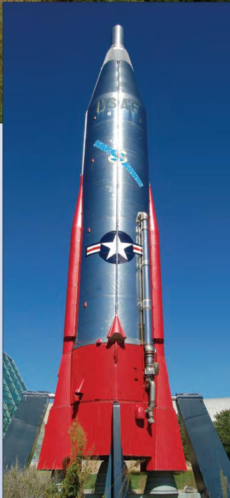
The Atlas D missile shown in the photograph is very similar in design to the next-generation Atlas E missiles which were deployed in the nine missile silos manned by the 548th Strategic Missile Squadron, based at Forbes Air Force Base at Topeka, Kan. The Atlas E was improved from the Atlas D with a more enhanced engine design and a small guidance computer. Atlas D missiles were also used in manned, earth-orbiting Mercury missions.
