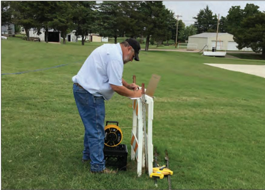
Geologist Ned Marks of Terrane Resources, Stafford, Kan., records water level measurement from nearby piezometer hole during pumping test.
