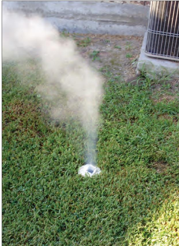
Smoke testing can help locate sources of infiltration and inflow. Smoke is emitting from an uncapped cleanout in the homeowner's service line. This same opening will also allow rainwater to enter.
