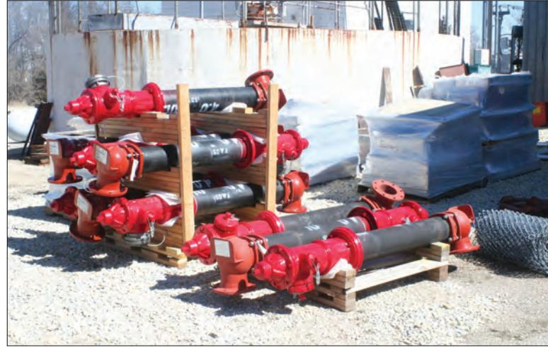
This photo shows the new fire hydrants after delivery to Enterprise. Note the “stortz” adapters installed on the 4.5 nozzles. These adapters speed fire department connection during fire response; they also have less friction loss than the standard threaded fittings.
