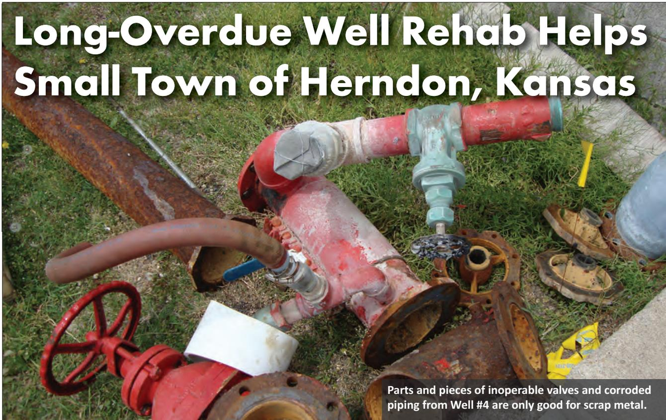
Parts and pieces of inoperable valves and corroded piping from Well #4 are only good for scrap metal.
