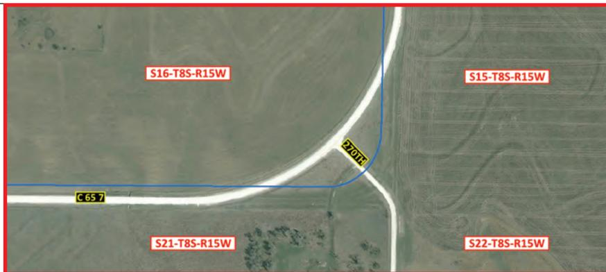
Graphic 2 displays the same intersection in an aerial photograph from 2009. The county has reconfigured the intersection; subsequently the RWD had to move its water line. This image shows the old location of the water line at the new intersection.
