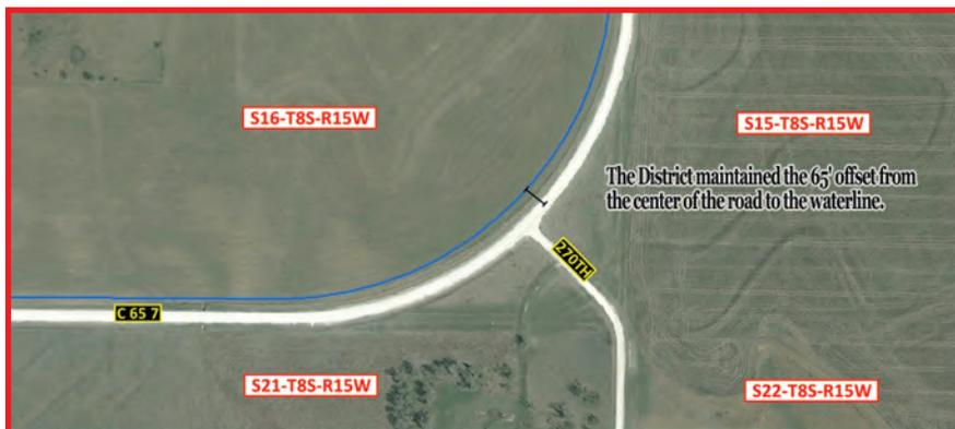
Graphic 3 reveals the updated location of the water line with the same 2009 aerial photograph. By keeping track of updates with GPS and measurements, future locating of pipelines will be much easier.
