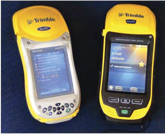
The Trimble GeoExplorer 6000 hand-held (shown on right) has a faster processor, greater memory, new operating system, built-in camera, floodlight technology (which allows better data collection in hills, trees or "urban jungles"), Wi-Fi, Bluetooth and available cellular modem which makes it superior to the previous 2005 GeoXH (on left).
