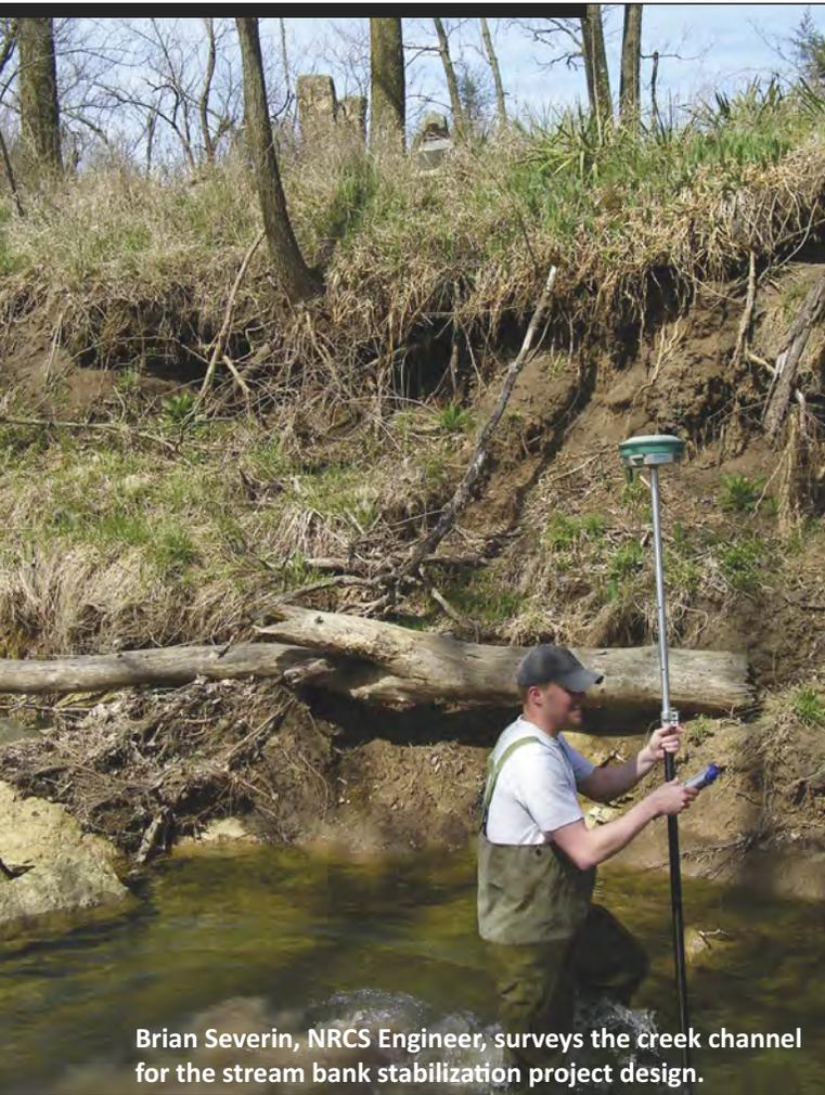
Brian Severin, NRCs Engineer, surveys the creek channel for the stream bank stabilization project design.
