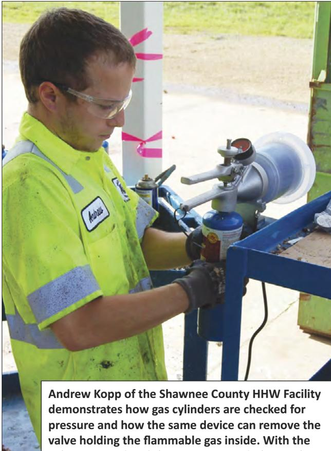
Andrew Kopp of the Shawnee County HHW Facility demonstrates how gas cylinders are checked for pressure and how the same device can remove the valve holding the flammable gas inside. With the valve removed and the gas evacuated, the steel cylinder can be safely recycled.
