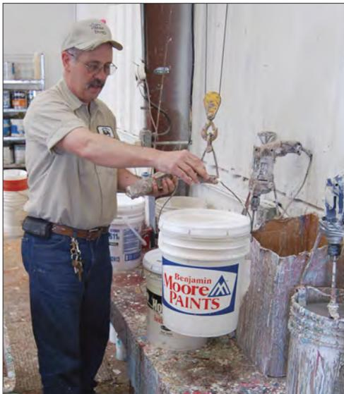
Eddie Spencer of the Shawnee County HHW Facility demonstrates how 5-gallon buckets of latex paint are moved from carts to the mixing table and back. The same device is used to lift the less than full buckets for pouring into buckets ready for mixing.
