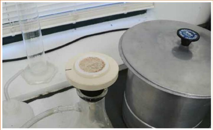
This photo shows the filter for a Total Suspended Solids (TSS) test after the sample was drawn through it. Both photos were taken in the city of Sabetha's wastewater treatment plant.
