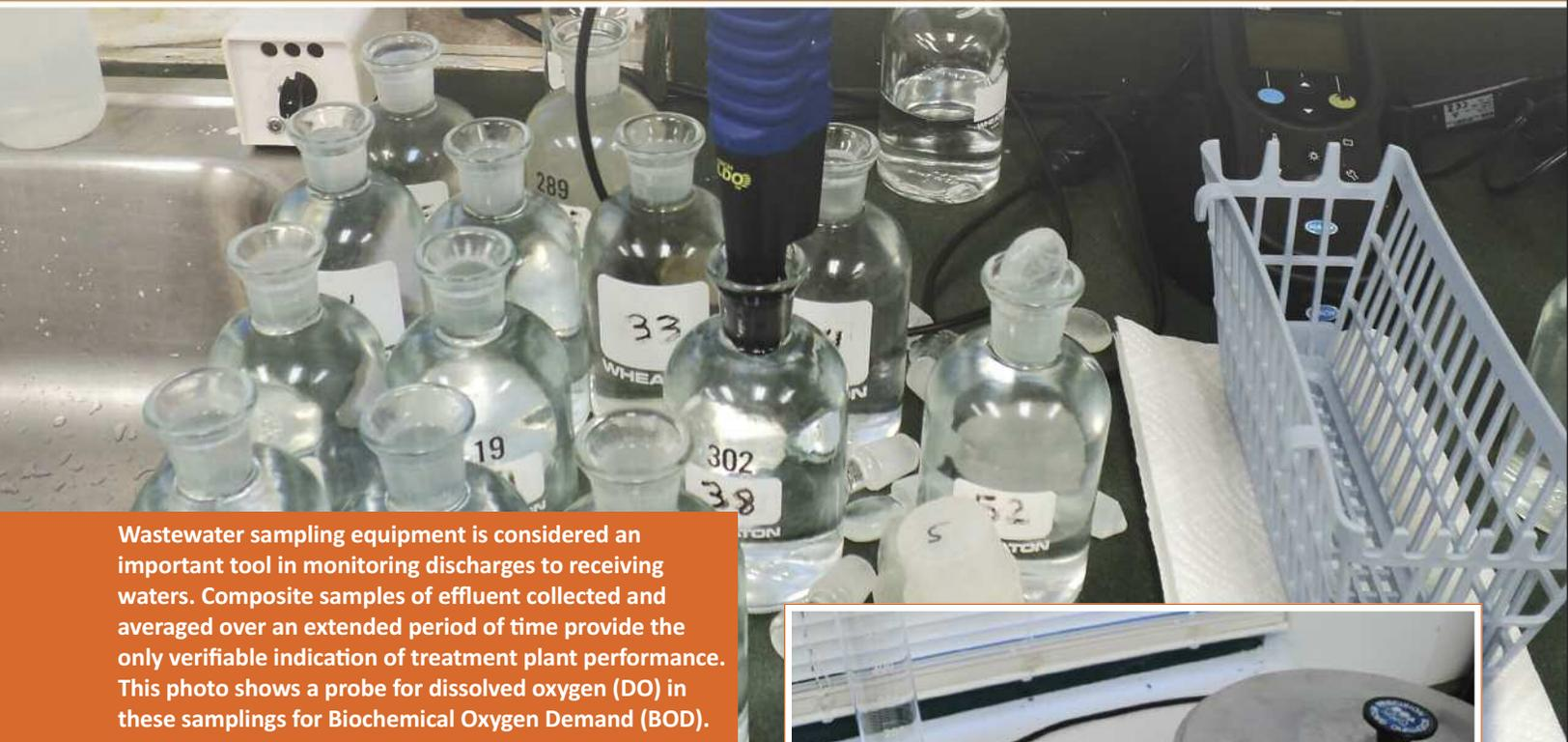
Wastewater sampling equipment is considered an important tool in monitoring discharges to receiving waters. Composite samples of effluent collected and averaged over an extended period of time provide the only verifiable indication of treatment plant performance. This photo shows a probe for dissolved oxygen (DO) in these samplings for Biochemical Oxygen Demand (BOD).
