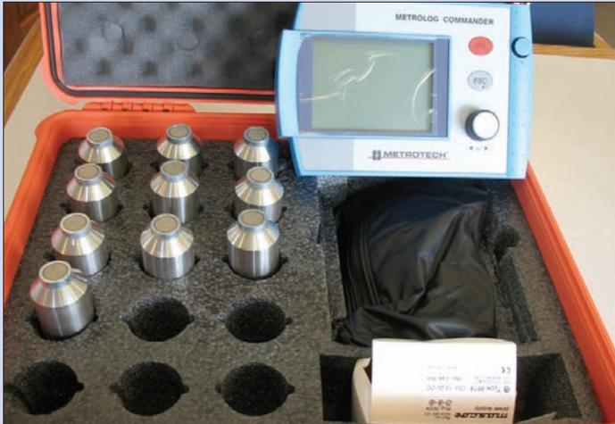
*This set of "data loggers" is but one of many devices KRWA uses to help locate water loss. The small cone shaped units are placed on valves, meter setters or any other part of the distribution system to detect system noise. Typically the units are programmed to turn on at 2 a.m. and then shut off at 3 a.m. The information from each unit is then downloaded into the Commander for analysis. Suspected leakage can then be investigated.*
