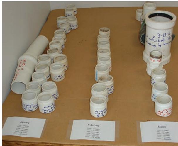
**Washington RWD 1 has been plagued by many problems with 1.5-inch, solvent weld PVC. The district tracks all repairs. In 2006, the district repaired 130 leaks; in 2010, the district repaired 129 leaks.**
