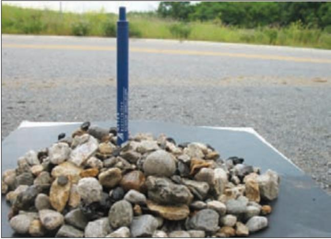
In addition to this pile of small rocks (see pen for comparison), other pieces of metal up to several inches long were trapped in front of another large meter screen. Obviously this new water system was not pigged. The probability of additional debris being in the system is very high.
