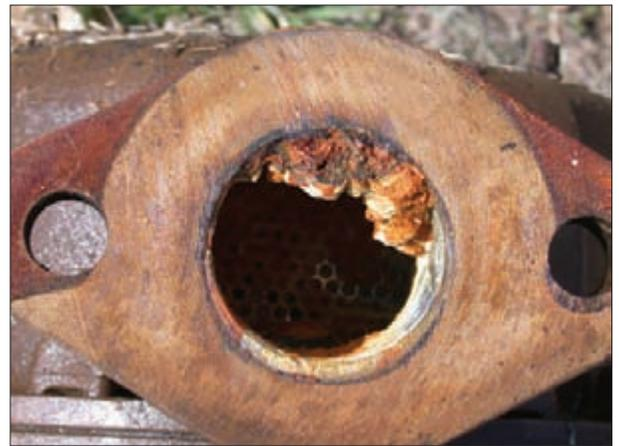
This meter was registering inaccurately. Highly mineralized water can cause buildups such as this inside meters. This meter had not been tested for fifteen years.
