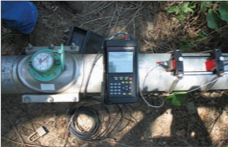
Use of a "non-intrusive meter", similar to that used by the Division of Water Resources to test raw water meters, is necessary when there is no test port available. In the test above, the pipe had full flow.
