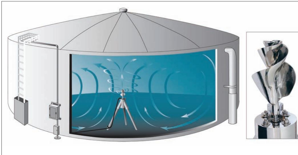
Figure 7: Diagram of a highly energy efficient active mixing system using biomimicry designed impeller (photo on right) to eliminate thermal stratification and achieve homogenous water chemistry.
