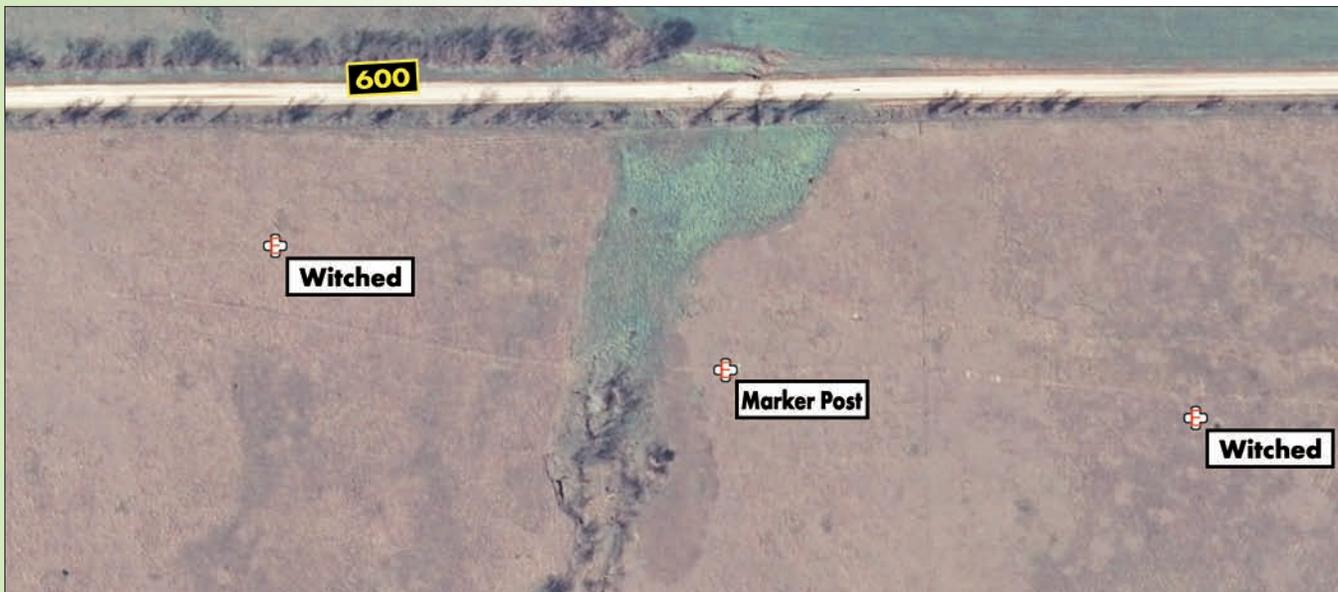
Graphic No. 1: A trench line is visible on this aerial. The red crosses are line points that were collected with a GPS coordinate based on the operator's instruction. The line point in the middle was collected at a waterline marker post; it is located directly over the trench line in the photo. The two line points on either side are identified as "witched" and it is obvious that the rods were not cooperating that day. So much for witching.
