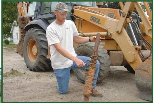
**Corroded steel pipe in Greenleaf, KS has had many repair clamps applied. This section of deteriorated pipe is an example of one such section. Superintendent Jerry Baker says it was a good visual aid when the city made application to KAN STEP for funding a new water system.**
