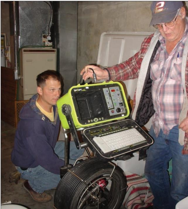
Fred Weins (plaid Jacket) and Tony Wedel of city of Moundridge set up a demonstration camera from Key Equipment to try to find cause of odor entering a residence. The city now owns a similar camera with 400 feet of cable and is equipped with a locator beacon to locate the head of cable; it can be used with the city's existing locator. In this case, the problem was failed glue joints on a vent pipe from an upstairs bathroom.
