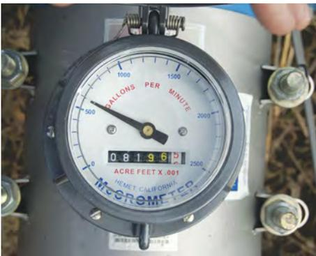
This photo shows the face of a typical irrigation water flow meter.
