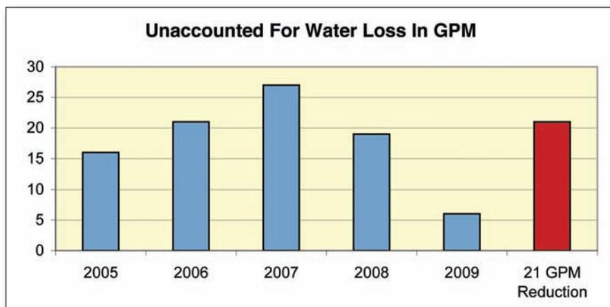
A water system in north-central Kansas was able to reduce its water loss from 27 gallons per minute in 2007 to 6 gallons per minute in January 2009. In the summer 2008 this system was losing 41 gallons per minute before two leaks were located and repaired.
