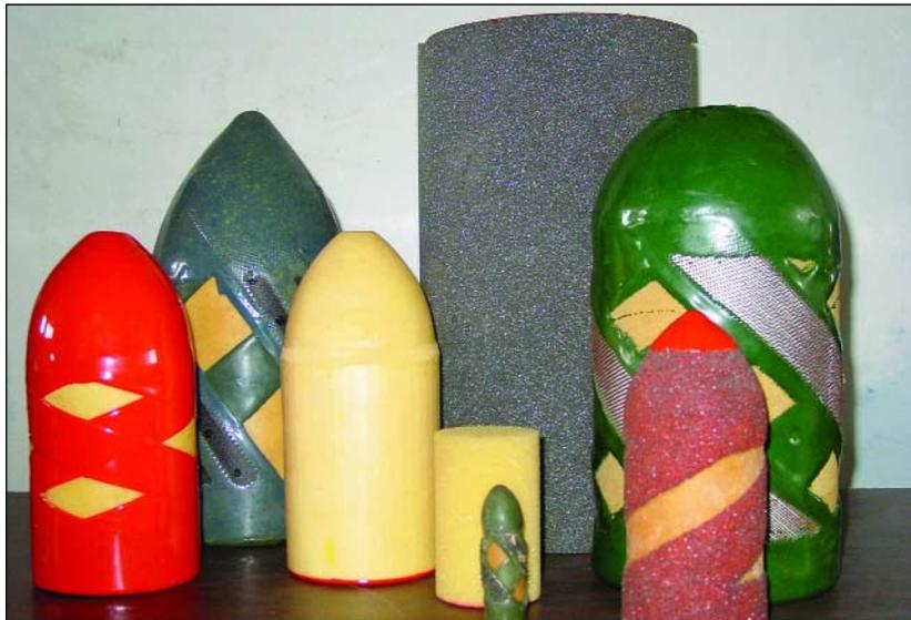
*This photo shows a sample of various poly pigs that KRWA keeps available for projects. The pigs can be fabricated for any pipe size. A variety of coatings can be applied, depending on the specific needs of the project involved.*
