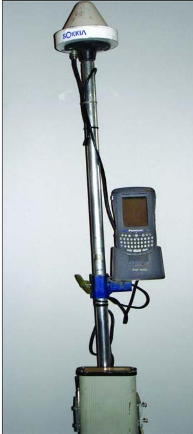
*This new handheld GPS data collector (below) replaces previous units that KRWA operated. As shown at left, those required an antenna, data logger and battery pack – all connected by wires.*
