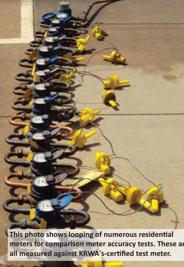
This photo shows looping of numerous residential meters for comparison meter accuracy tests. These are all measured against KRWA's-certified test meter.
