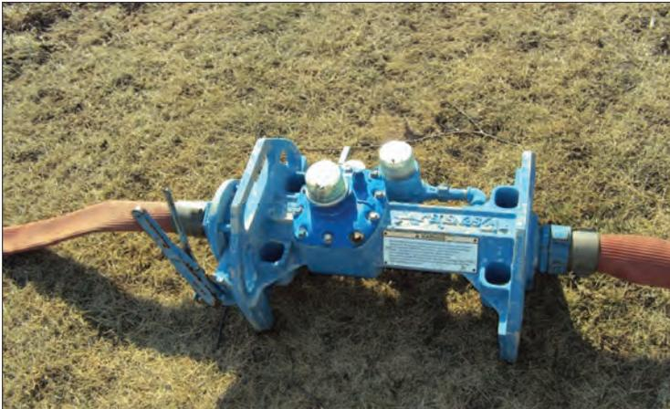
KRWA has four units similar to this 4-inch meter. This size unit is typically used to test meters up to 500 gpm. KRWA also utilizes several non-intrusive meters for higher flow rates.
