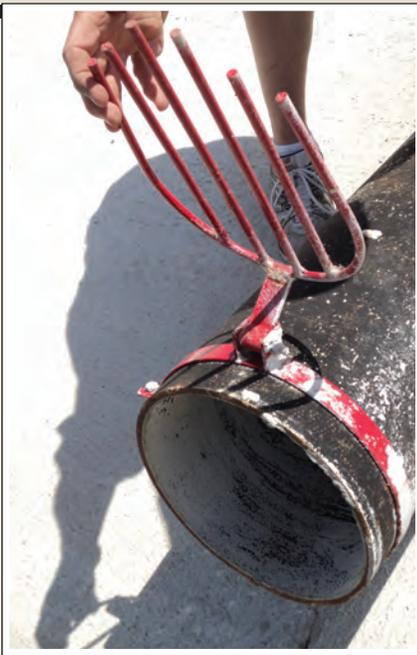
**An ideal type of turtle guard allows any debris that may accumulate to drop off the end.**
