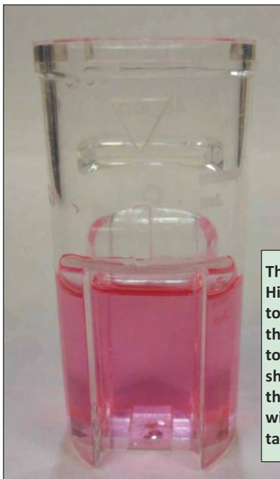
The plastic vial is only used in High Range. The vial is filled to the 5-ml mark. Also note the raised triangle near the top of the vial. This triangle should be facing away from the keypad before covering with the instrument cap and taking readings.
