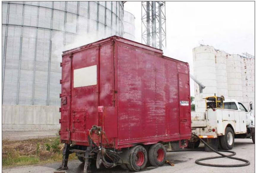
This “steam trailer” contains equipment to heat rolls of material to reline pipelines. Steam hose attached and steaming coil of pipe inside steam trailer.
