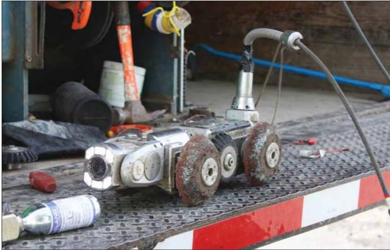
This self-propelled robotic cutting device is used to cut the service taps back into the sewer pipeline after relining, making the project something akin to a non-invasive surgery.
