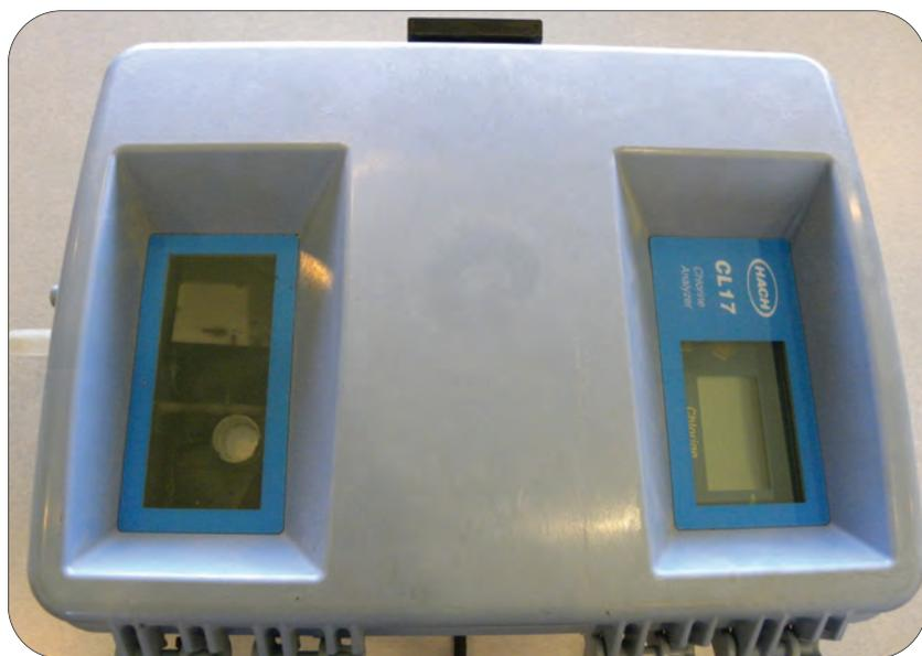
**The Hach CL17 Analyzer is a microprocessor-based analyzer designed to monitor a sample stream continuously for chlorine content.**
