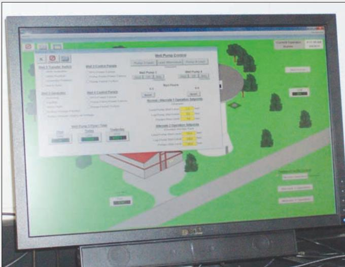
The SCADA system provides various alarms and online monitoring for turbidity, chlorine and pH.
