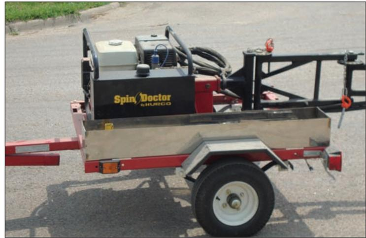
This Hurco Spin Doctor valve exerciser owned by the city of Washington, KS was originally designed to mount in a truck receiver hitch with the power unit loaded in the bed. Because loading required three or four people then City Water, Wastewater and Street Supervisor Greg Metz and other crew members constructed a small trailer to transport the equipment. The city invested \$300; a trailer could have been purchased for an additional \$2,500.
