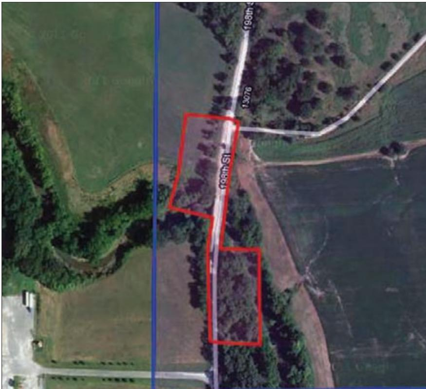
The locate request for this call was specific to be a five-foot radius at two points: 1) “at the white flag at 1,723 feet from the intersection to the south”; and, 2) “at the white flag at 2,178 feet from the intersection.” Again, the polygons drawn by the Kansas Call Center includes both sides of the road and extensive additional areas.
