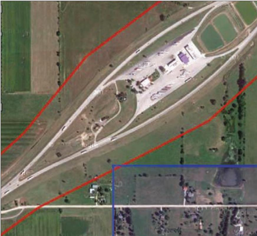
The red-lined area shows the polygon that the Kansas Call Center operator generated for a recent locate request. The blue line is the limit of the polygon for a rural water district in that area. The important issue with this locate is that the excavator's specific request according to the ticket issued, was for locations within the limits of the road right of way. The One-Call polygon (red) is clearly hundreds of feet beyond the request and as a result, forced another wasted ticket to the RWD.
